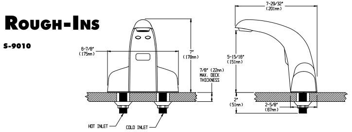
NOTE: Unless otherwise specified, all inlets are sized for either coupling or sweat connections. Unless otherwise specified, all dimensions are in inches and are subject to change without notice. Position faucet as close to the edge of the sink as possible.
