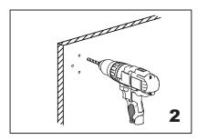
Drill 3/16" holes, make sure to keep drill level
