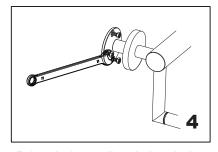
Driver bolt nut directly into holes
