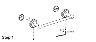
Loosen the set screw on the accessory and remove the backing plates. Position the accessory against the wall and mark outline with pencil.
